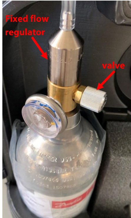
Illustration 74: Fixed flow regulator with valve connected to calibration gas cylinder
