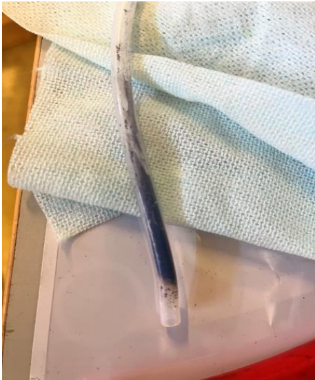
Soot in the air hose
