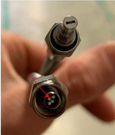
4 out of 6 fibers are working
