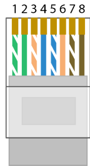
Illustration 28: Example of RJ-45 connector with wire assignment TIA 568 A
